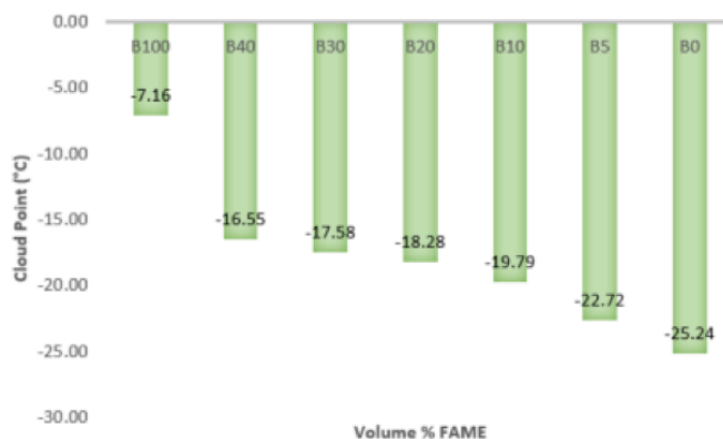
Figure 5. Cloud point as function of % FAME in various biodiesel-conventional diesel blends.
